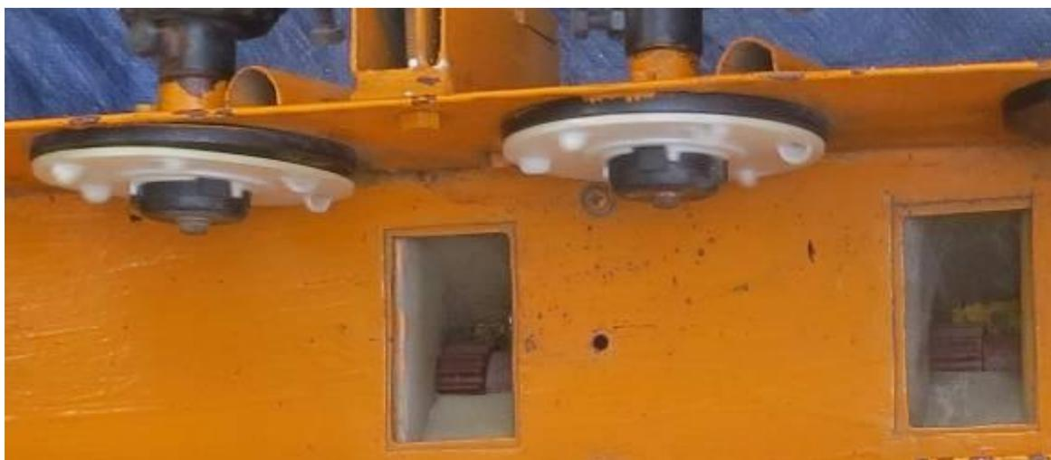
The VMP now has both the fluted roller seed meters ( for planting of cereals such as wheat and rice) and inclined plate seed meters (similar to the Earthway design) for spaced plants such as maize.
