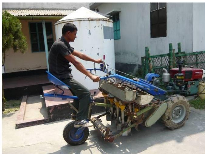
The Version 9 (left) has the dual type seed meters ( as shown below) whilst the Version 10 ( right) has a seat fitted.
