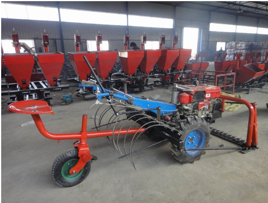
Two wheel tractor with sickle bar mower and hay rake These options below may offer alternatives.
