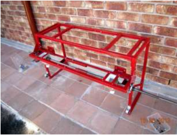
The basic frame (left) with the fertiliser meters. An overall view of the unit (right) showing the vertical spoon feed metering system and the fertiliser boxes. No down tubes or drive chains have yet been fitted. Note the 'temporary' seed boxes on the top of the seed drill.
