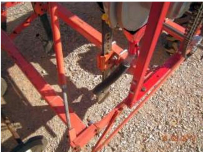
The seed delivery tube from the meter to the tine is shown on the left. If required, the tine can be removed, and a disc opener used as an alternate soil engaging tool. The picture on the right shows the frame 'flat packed' for transport to Africa.
