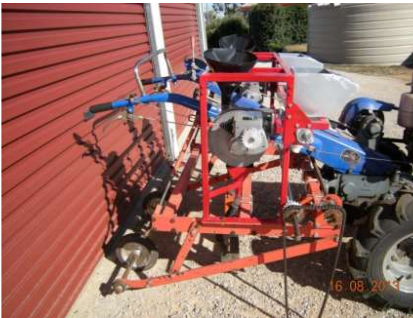
These views show more of the detail. The drive from the ground wheel goes to the original countershaft above the front tool bar. This further drives to a lay shaft immediately behind the front countershaft, and then to the vertical spoon feed meters. This set-up allows a variety of sprocket sizes to be used for maximum flexibility in choice of seed and fertiliser rates.
