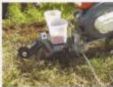
FIGURE 3. Prototype no-till planter (John Morrison, University of Texas) on trial in Tanzania. Photo: Peter Chisawillo.
