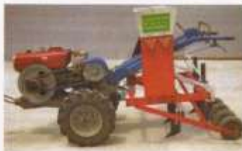
FIGURE 2. ARC Gongli no-till planter for 2WTS. Photo: ARC Gongli seed drill instruction manual.
