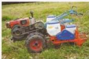
FIGURE 11. Two Knapik no-till planter units attached to a 2WT. Photo: Brian Sims
