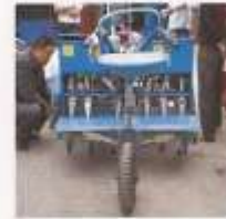
FIGURE 8. Full width rotary seeder / fertilizer modified for strip till sowing. Photo: Ken Sayre.
