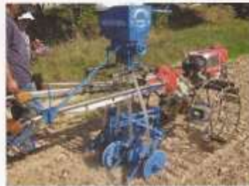
FIGURE 6. Thai Department of agriculture designed no-till drill for dry direct seeding of rice. Photo: Jack Desbailles.
