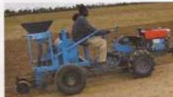
FIGURE 4. Ndume no-till planter and sprayer mounted on a Kungfu 2WT. Photo: Brian Sims.
