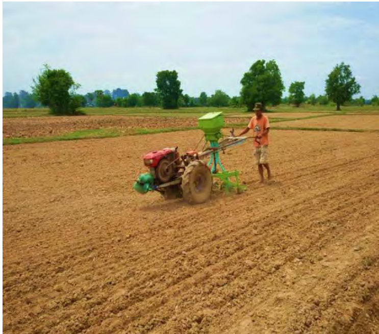
Direct seeding of rice in Laos, using a Thai made seed drill.
