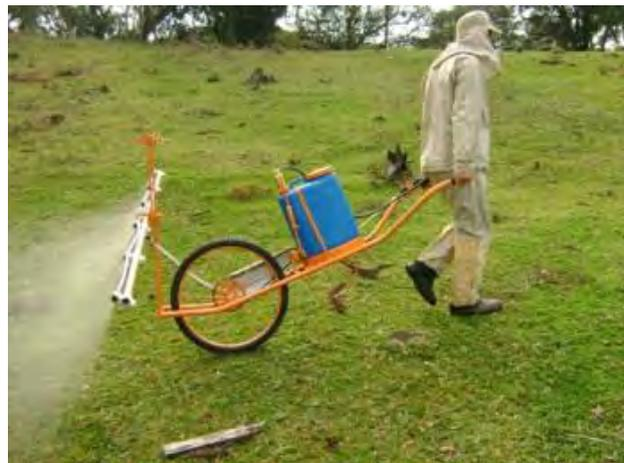
The sprayer on the left was fabricated by Joseph Mutua (KENDAT Kenya) and a wheel barrow model on the same principle is shown on the right. A ground wheel drives the hand pump via a chain and pitman arm.
