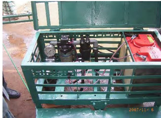
This Bangladeshi one is a trailing 8 nozzle unit. It has a 12V diaphragm pump, 150 litre tank, and is on 800mm track. It is powered by an automotive battery which has to be re-charged every few hours. It has a locally made folding boom.
