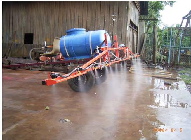
This trailing unit was made in Cambodia in co-operation with CIRAD. It has a centrifugal pump close coupled to a small petrol motor. It has a 10 nozzle Australian made boom, and a locally sourced 300 litre tank.
