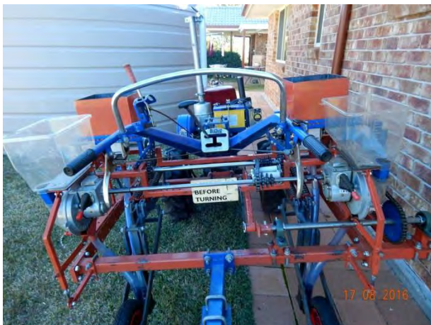
View from the seat showing seed & fertiliser boxes (left). The rope trip lift (right)
