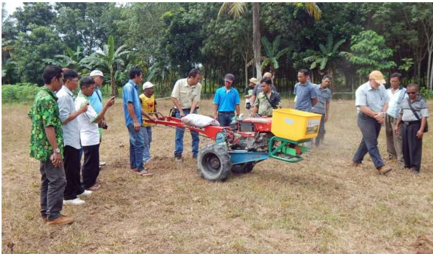
The 'Quick' 8.5HP 2WT being demonstrated with a front mounted fertiliser broadcaster.
