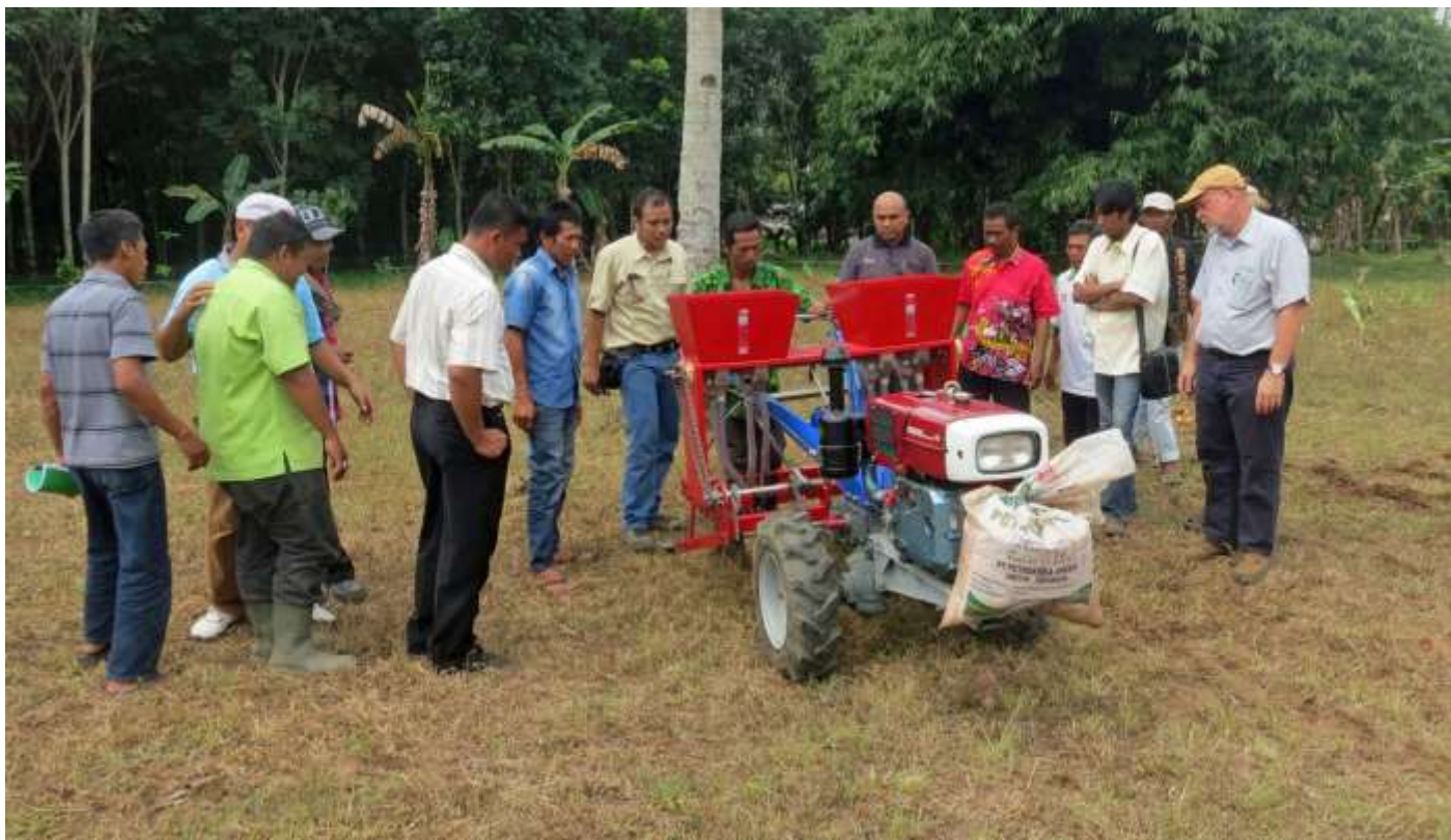
Participants operate the ARC Gongli in the field (note zero tillage- field previously sprayed with Roundup)
