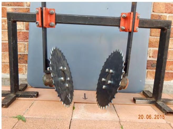
The laser cut discs (left) and the discs set up for operation as angled single disc openers for the Gongli Africa 2 seed drill (right).
